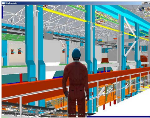
Figure 1: A screenshot extracted from a VR prototype showing the avatar inside one of the main facilities in the pelletizing plant.
